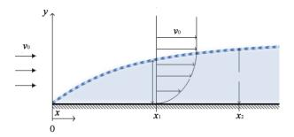
If the boundary layer is taken into account in the computation no-slip Boundary Condition is used:  $\mathbf{v}_{Wall} = \mathbf{0}$ . If boundary layer is not considered  $\Rightarrow \mathbf{v}_{Wall} = \mathbf{v}_{Slip}$
