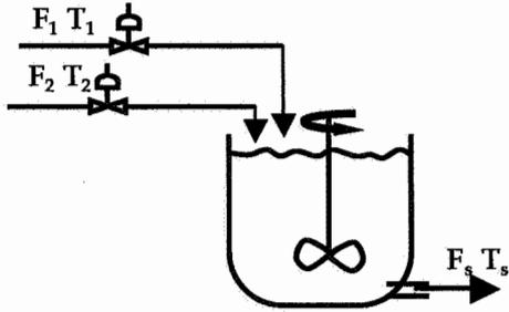
$$\begin{bmatrix} F_s(s) \\ T_s(s) \end{bmatrix} = \begin{bmatrix} \frac{e^{-5s}}{15s+1} & \frac{e^{-5s}}{15s+1} \\ -\frac{1.3e^{-15s}}{60s+1} & \frac{2e^{-15s}}{60s+1} \end{bmatrix} \begin{bmatrix} F_1(s) \\ F_2(s) \end{bmatrix}$$
