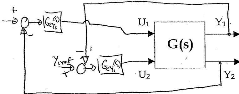
$$K = \begin{bmatrix} 1 & 2 \\ 1 & 1 \end{bmatrix} \quad \Delta = K \otimes (K^{-1})^T = \begin{bmatrix} -1 & 2 \\ 2 & -1 \end{bmatrix}$$
