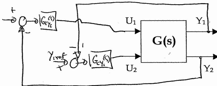
$$K = \begin{bmatrix} 1 & 2 \\ 1 & 1 \end{bmatrix} \quad \Lambda = K \otimes (K^{-1})^T = \begin{bmatrix} -1 & 2 \\ 2 & -1 \end{bmatrix}$$
