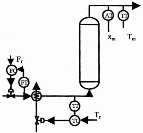
$$\begin{bmatrix} T_m(s) \\ x_m(s) \end{bmatrix} = \begin{bmatrix} \frac{-3.4e^{-1.93s}}{1.15s+1} & \frac{1.1e^{-3.70s}}{0.14s+1} \\ \frac{2.2e^{-0.65s}}{1.34s+1} & \frac{-0.8e^{-6.15s}}{1.27s+1} \end{bmatrix} \begin{bmatrix} F_r(s) \\ T_r(s) \end{bmatrix}$$
