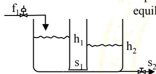
$$0 = f_{10} - s_{10}\sqrt{2g(h_{10} - h_{20})} \quad f_{10} = f_{1-20}$$
