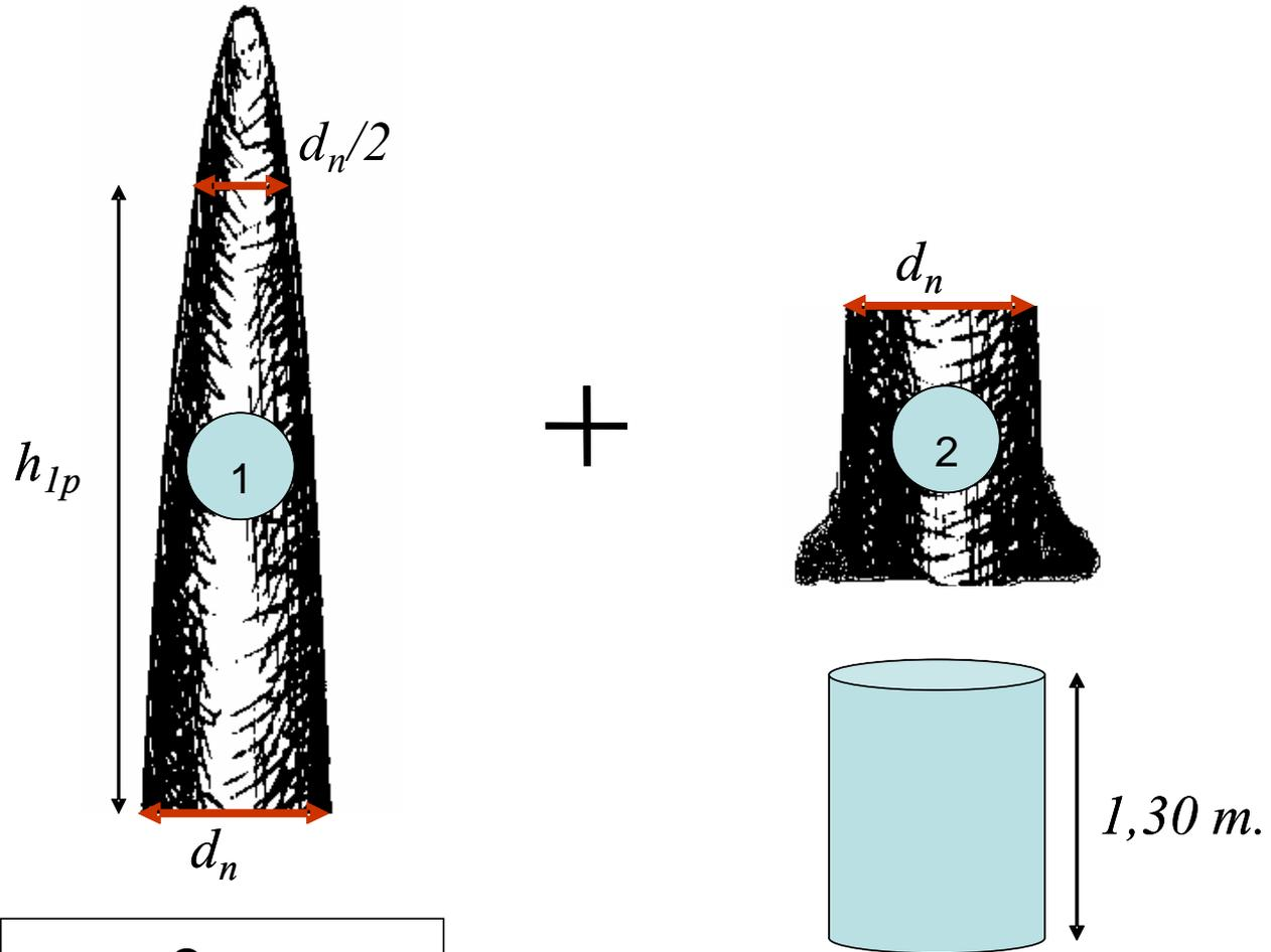
$$V_{real} = V_1 = \frac{2}{3} S_n \cdot h_{1p} + V_2 = S_n \cdot 1,30$$
