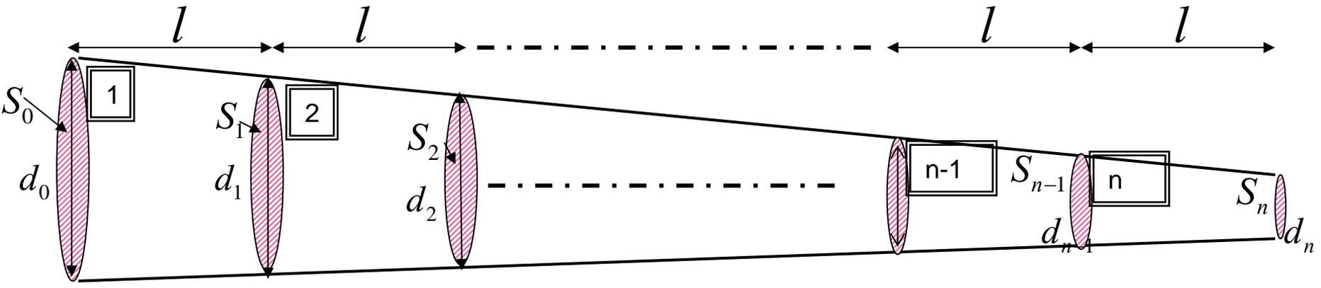
$$S_0 = \frac{\pi}{4} \cdot d_0^2 \quad S_1 = \frac{\pi}{4} \cdot d_1^2 \quad S_2 = \frac{\pi}{4} \cdot d_2^2 \quad \dots \quad S_{n-1} = \frac{\pi}{4} \cdot d_{n-1}^2 \quad S_n = \frac{\pi}{4} \cdot d_n^2$$
