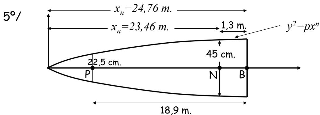
$$\left\{ \begin{array}{l} N \rightarrow 22,5^2 = p \cdot 23,46 \\ B \rightarrow \left(\frac{d_B}{2}\right)^2 = p \cdot 24,76 \end{array} \right\} \Rightarrow \left\{ \frac{\left(\frac{d_B}{2}\right)^2}{24,76} = \frac{(22,5)^2}{23,46} \right\} \Rightarrow d_B = 46,23 \text{ cm.}$$
