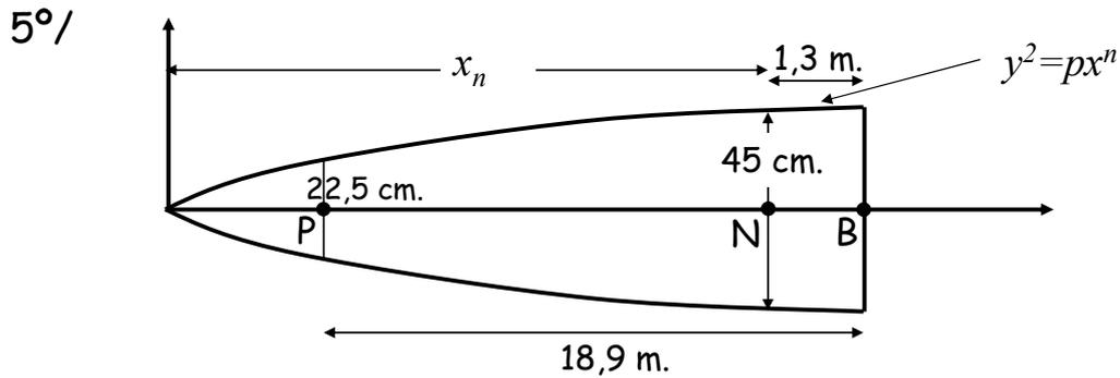
$$\left\{ \begin{array}{l} N \rightarrow 22,5^2 = p \cdot x_n \\ P \rightarrow \left(\frac{22,5}{2}\right)^2 = p \cdot (x_n + 1,3 - (18,9)) \end{array} \right\} \Rightarrow \left\{ \frac{22,5^2}{x_n} = \frac{(11,25)^2}{(x_n - 17,6)} \right\} \Rightarrow$$
