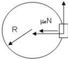
$$\begin{aligned}\mu_e N &= ma_n = m \frac{v^2}{R} \\ N - mg &= 0\end{aligned}$$
