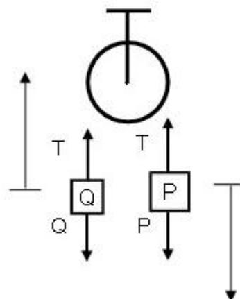
$$\left. \begin{array}{l} P - T = \frac{P}{g}a \\ T - Q = \frac{Q}{g}a \end{array} \right\} \Rightarrow a = \frac{P-Q}{P+Q}g \Rightarrow v = \frac{P-Q}{P+Q}gt \rightarrow s = \frac{1}{2} \cdot \frac{P-Q}{P+Q}gt^2$$
