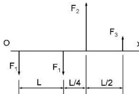
DATOS:  $F_1 = 18 \text{ N}$   $F_2 = 18 \text{ N}$   $F_3 = 15 \text{ N}$   $L = 66 \text{ m}$
