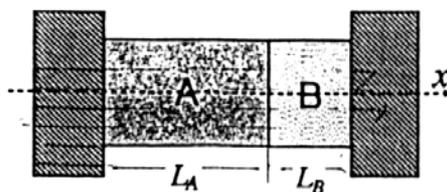
**Datos:**  $L_A = 2L_B = 2\text{cm}$ ;  $E_A = 2E_B = 200\text{GPa}$ ;  $\nu_A = \nu_B = 0,25$ ;  $\alpha_B = 2\alpha_A = 10^{-5} (\text{°C})^{-1}$ .
