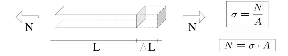
DESIGN TENSION RESISTANCE (  $\sigma = f_{yd}$  )  $N_{Rd} = f_{yd} \cdot A = \frac{f_y}{\gamma_M} \cdot A$
