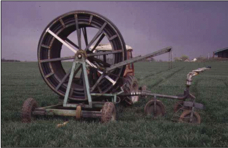
Figure 2.37: Example of a raingun [220, UK, 2002]
