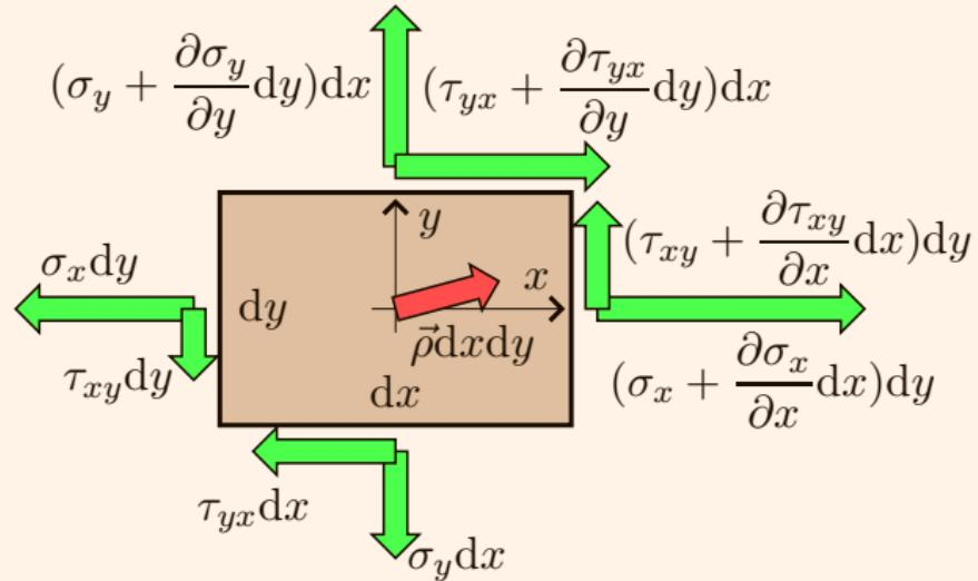
$$\sum F_x = 0 \Rightarrow \frac{\partial \sigma_x}{\partial x} + \frac{\partial \tau_{yx}}{\partial y} + \rho_x = 0 \quad \sum F_y = 0 \Rightarrow \frac{\partial \tau_{xy}}{\partial x} + \frac{\partial \sigma_y}{\partial y} + \rho_y = 0$$
