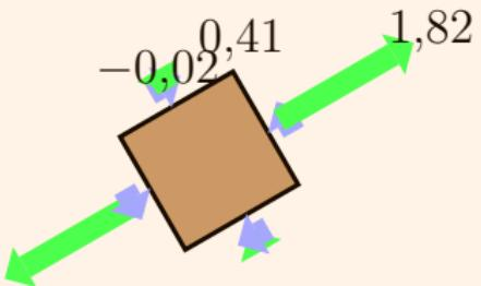
$$\begin{aligned}\sigma_n &= \sigma_x \sin^2 \alpha + \sigma_y \cos^2 \alpha - 2\tau_{xy} \cos \alpha \sin \alpha \\ &= -0,02\end{aligned}$$
