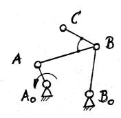
Find a loop line "∞" as coupler curve of point C by using SAM 6.0
