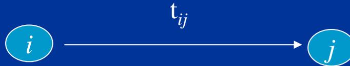
$$t_j = \text{máx}(t_i + t_{ij}), \forall i$$
