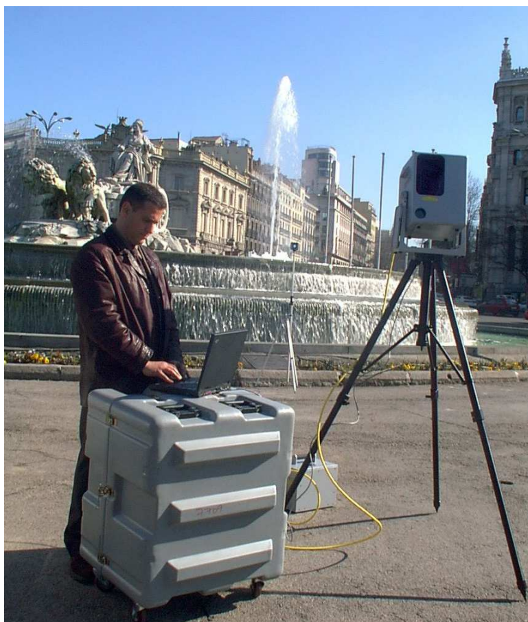
Illustration 10: Equipment Cyrax 2500 by Leica
