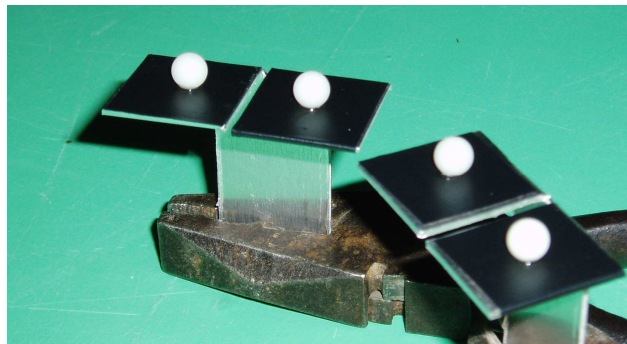
Figure 8: Sighting points for the topographical grid and pretargeting
