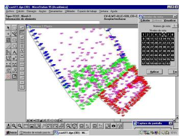
The *dxf* files were imported using CAD *Microstation* and the data was separated with different levels and colours, in such ways that later when mistakes were detected, it was possible to separate that series of data. The different points defining the upper and lower outlines were then joined up, as well as the vertical lines. In this manner the floor of the archaeological building was defined as well as the 3D structural outlines.
