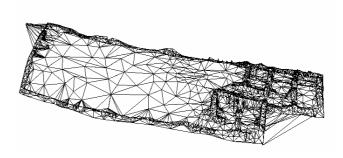
Once the mesh was separated into different layers using *AutoCAD*, the file was reconfigured in order to use *3D Studio Max* program.
