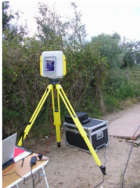
Figure 10: data acquisition in the basilica with laser scanner
