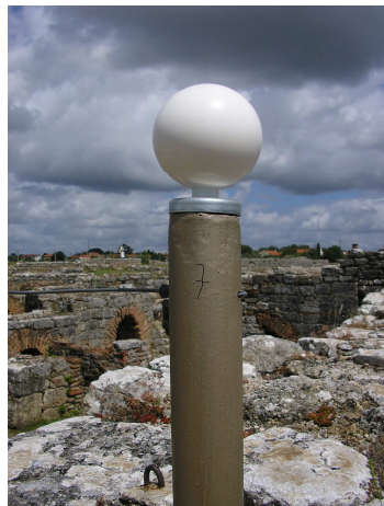
Figure 9: Spheres used for the georeferenciation
