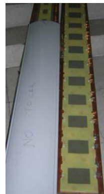
Base station antennas for mobile systems applications: GSM 1800 MHz: Vertical pol.° sectorial 65° & 90° antennas
