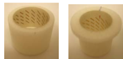
Circularly Polarized Omnidirectional Millimeter Wave Monopole with Parasitic Strip Elements for Identification Friend or Foe System
