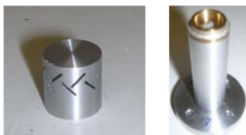
Omnidirectional Circularly Polarized Slot Antenna Fed by a Cylindrical Waveguide for Identification Friend or Foe System in the 37GHz band
