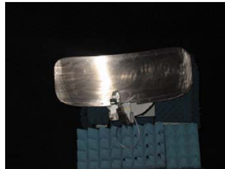
Antenna for satellite communication from a high speed train
