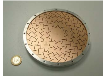
Antenna for TV reception via satellite (DBS) at 12 GHz
