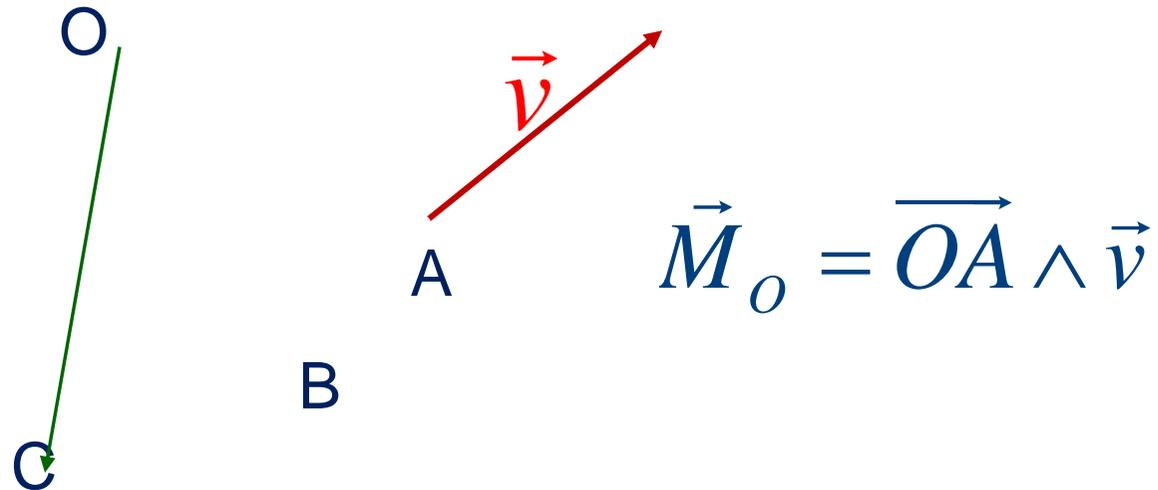
$$\vec{M}_C(\vec{v}) = \overrightarrow{OA} \wedge \vec{v} = (\overrightarrow{OC} + \overrightarrow{CA}) \wedge \vec{v} = \overrightarrow{OC} \wedge \vec{v} + \overrightarrow{CA} \wedge \vec{v}$$
