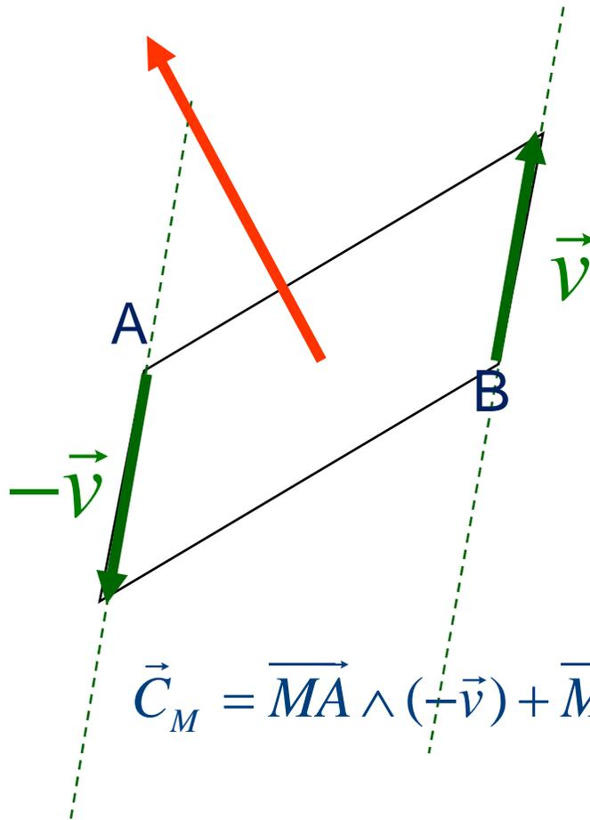
$$\vec{C}_A = \overrightarrow{AA} \wedge (-\vec{v}) + \overrightarrow{AB} \wedge \vec{v} = \overrightarrow{AB} \wedge \vec{v}$$
