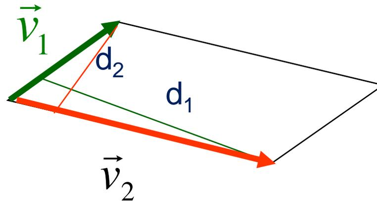
$$Area = |\vec{v}_1 \wedge \vec{v}_2| = |\vec{v}_1| |\vec{v}_2| \text{sen } \varphi = |\vec{v}_1| d_1 = |\vec{v}_2| d_2$$
