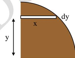
$$x_G = y_G = \frac{1}{M} \iint_A y dm = \frac{1}{M} \iint_A y \sigma x dy = \frac{\sigma}{M} \int_0^{\pi/2} R \sin \varphi R \cos \varphi R \cos \varphi d\varphi$$
