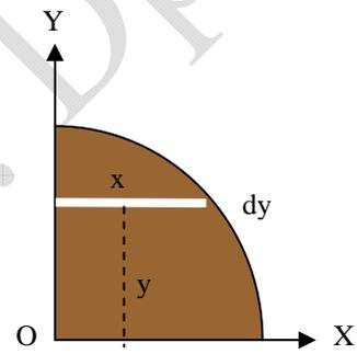
$$I_{OX} = \iint_A y^2 dm = \iint_A y^2 \sigma x dy = \sigma \iint_A (R^2 \sin^2 \varphi)(R \cos \varphi) R \cos \varphi d\varphi = \sigma R^4 \int_0^{\pi/2} \sin^2 \varphi \cos^2 \varphi d\varphi$$
