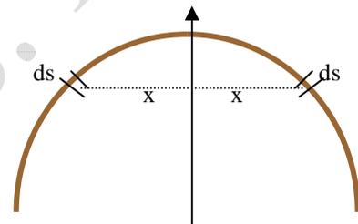
$$I_{OY} = \int_L x^2 dm = \int_L x^2 \lambda ds = 2\lambda \int_{L/2} (R^2 \cos^2 \varphi) ds = 2\lambda R^2 \int_0^{\pi/2} \cos^2 \varphi R d\varphi = 2\lambda R^3 \int_0^{\pi/2} \cos^2 \varphi d\varphi$$
